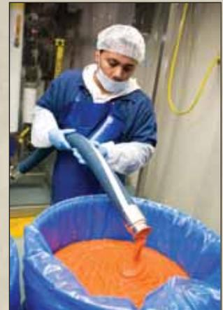
**Left, trailer-lift system for unloading fresh carrots. Right, pureed carrots, that have been sanitized, chopped and pasteurized, are filled into drums in the HEPA-filtered clean room.**
